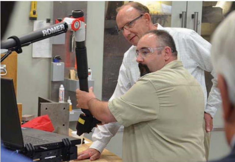
Mark Vance, advanced technical specialist at Clinkenbeard, demonstrates the capabilities of the Romer Absolute Arm.
